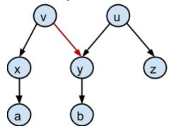
Figure 1: A new edge is created from vertex *v* to vertex *y*. Since vertices *x* and *y* belong to the same category, they must be merged.
