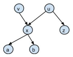
Figure 2: After the merging of *y* into *x*. It is possible that vertices *a* and *b* may need to be merged, but vertices *x* and *z* will never need to be merged.
